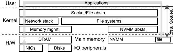
Figure 1: Today’s OS organization: No integration between network stack and NVMM abstractions. A light gray arrow indicates path of data from NIC to NVMM.
