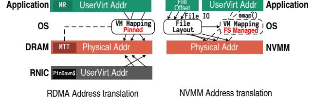
Figure 1: **Address translation for RDMA and NVMM.** RDMA (left) uses NIC-side address translation with pinning, while NVMM (right) allows the file system to maintain the layout of a file mapped to user address space.
