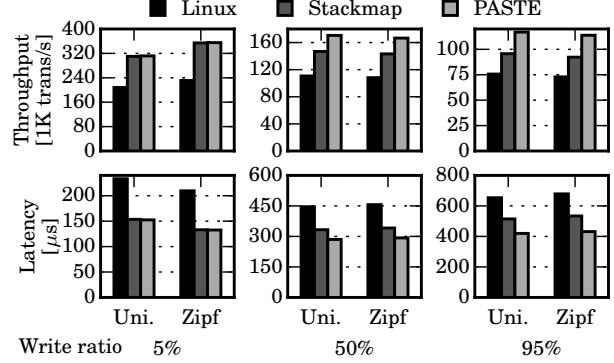
Figure 8: **Throughput and mean latency with pKVS.** Latency plots have standard deviations at most 30 % (Linux), 17 % (StackMap) and 11 % (PASTE).
