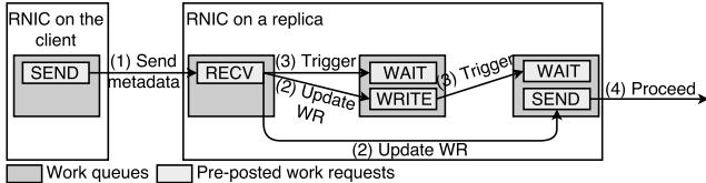
**Figure 7: Datapath of gMEMCPY primitive.**
