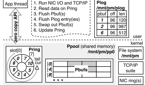
Figure 3: PASTE architecture: Packet buffers are named by a file backed by NVMM and pointed to by private application metadata.
