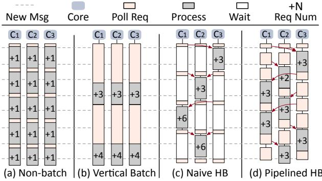
**Figure 4.** Sequence Diagram of Different Execution Model (gray dashed line indicates a new request arrives, “+N Req Num” means N of requests are batched together for persistence, red arrow means the action of stealing).
