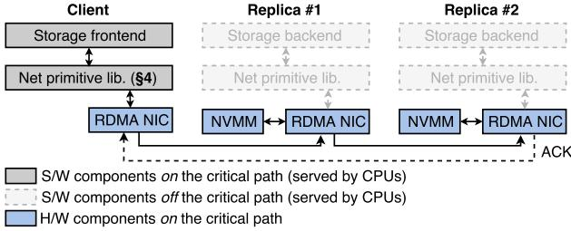
**Figure 3: Storage system architecture with HyperLoop.**
