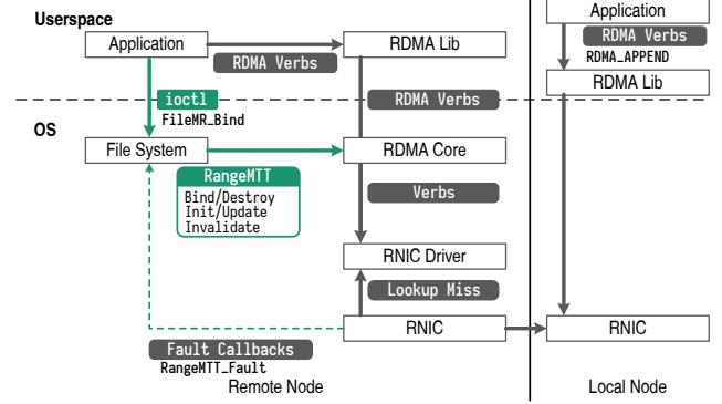
Figure 4: **Overview of FileMR components.** Implementing FileMR requires changes in file system, RDMA stack and hardware.
