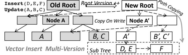
**Figure 5.** Overall Multi-version Data Structure
