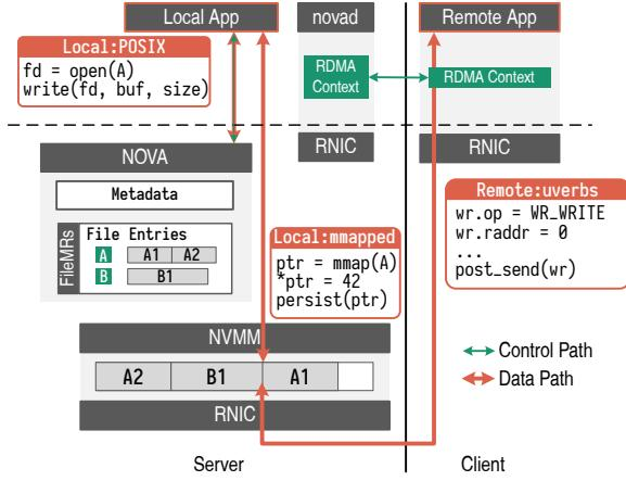
Figure 5: **Enabling remote NOVA accesses using FileMR.**
