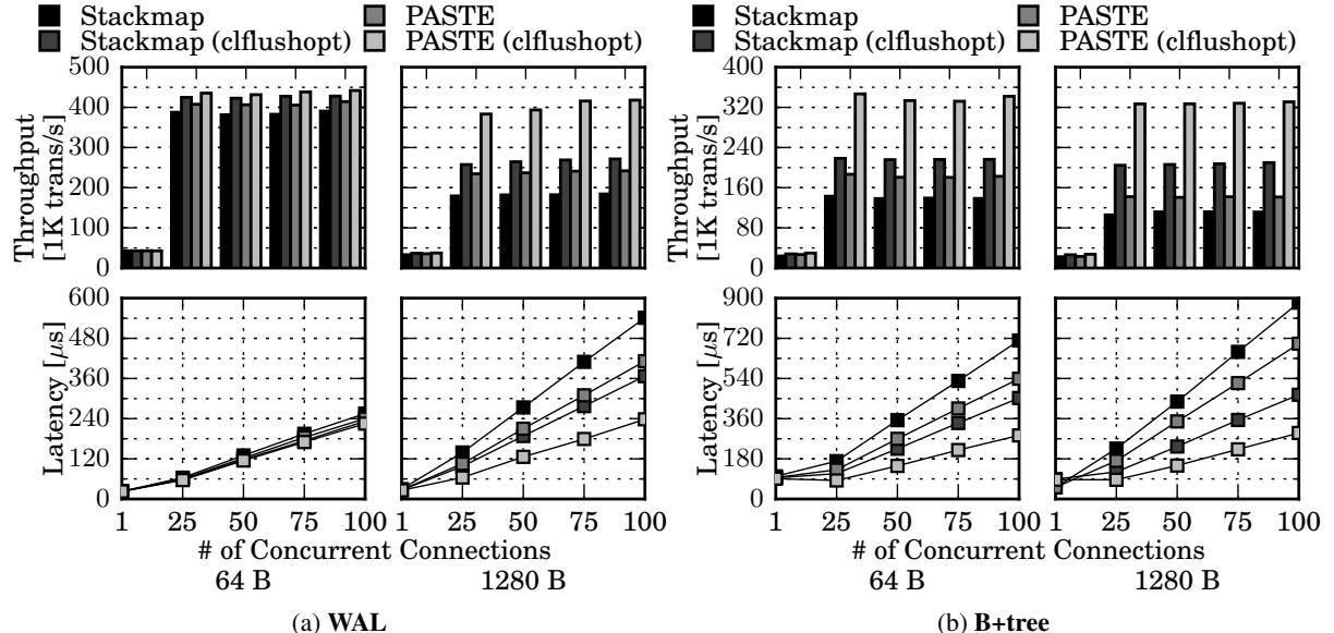
Figure 13: Throughput and mean latency with clflushopt.
