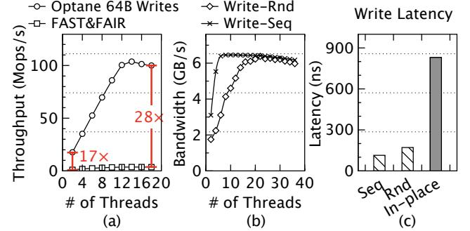
**Figure 1.** Performance Evaluation of Intel Optane DCPMM.
