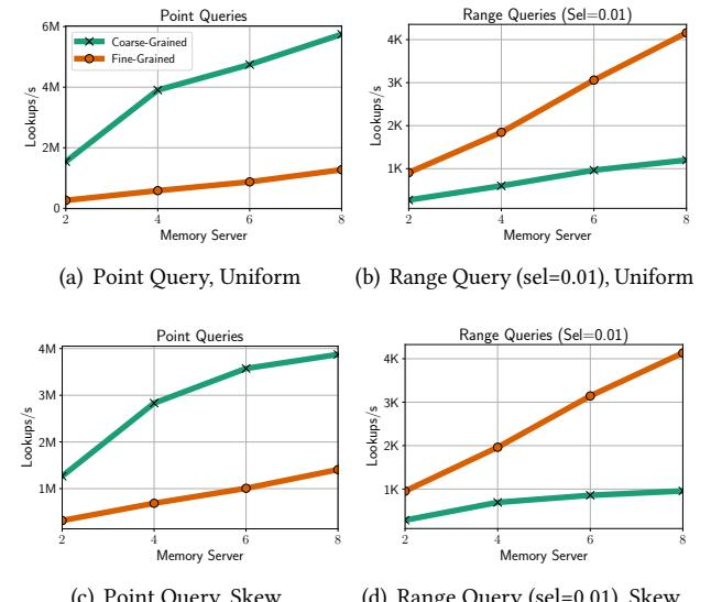
**Figure 11: Varying # of Memory Servers for Workloads A and B (Size 100M, 120 Clients)**
