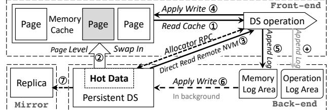
**Figure 4.** AsymNVM Framework Data Access Workflow
