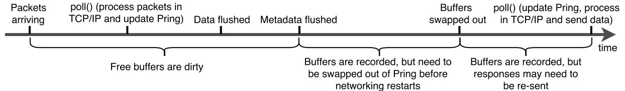
Figure 12: Buffer state over a networking event cycle.
