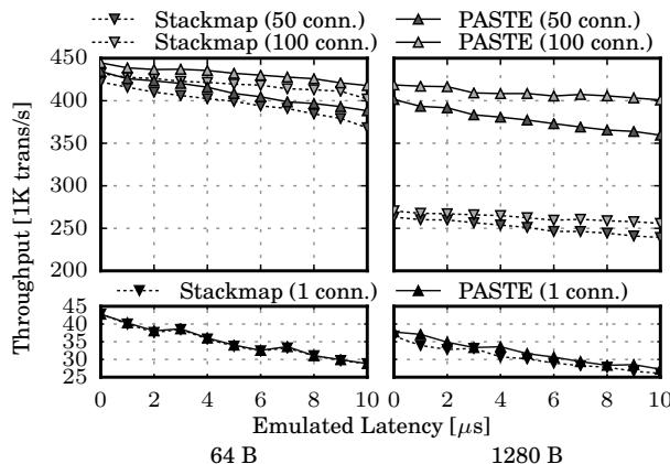
Figure 14: WAL throughput over emulated NVMM access latency.
