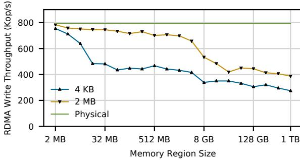
Figure 2: **RDMA Write performance over different memory region sizes.** This figure shows the throughput of 8-byte RDMA writes affected by the pin-down cache misses. Data measured on Intel Optane DC Persistent Memory with an Mellanox CX-3 RNIC.
