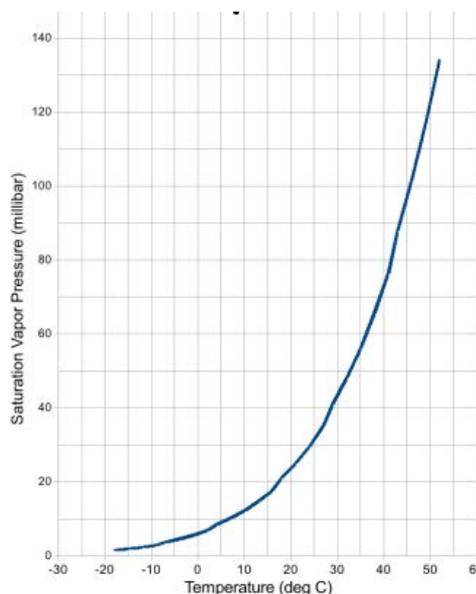
**Figure 1-6.** Air – saturation vapor pressure (According to The Engineering ToolBox)
