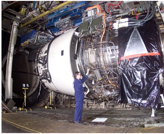
Fig. 13. Overhauling on a RR-Trent-900 jet engine ( Wiki ).
