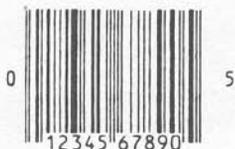
(UPC) found on most grocery store products (Figure 17-6). A photoelectric cell detects the pattern of absorbed and reflected light, converting it into a pattern of electrical signals, which operate the cash register and change inventory records. Many libraries use similar systems to maintain lender records and book inventories.
