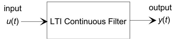
A LTI filter is dynamical SISO (single-input single-output) linear system, governed by an ODE with constant coefficients. From elementary linear system theory, some fundamental properties of LTI systems are:
