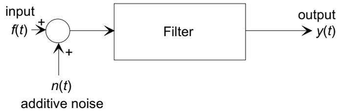
The task is to design a filter that will minimize the effect of the interference while not destroying information from the experiment.
