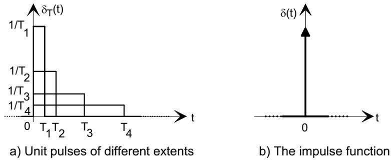
The figure below shows a *unit pulse* function  $\delta_T(t)$ , that is a brief rectangular pulse function of extent  $T$ , defined to have a constant amplitude  $1/T$  over its extent, so that the area  $T \times 1/T$  under the pulse is unity:
