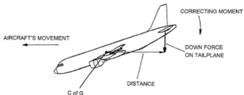
**Figure 4-17.** Longitudinal stability
