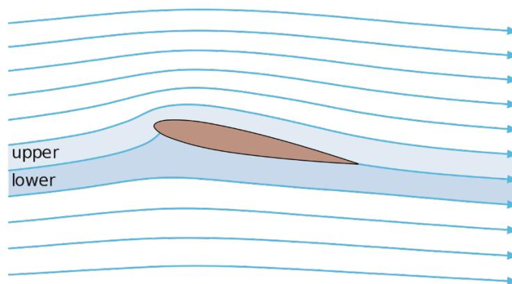
**Figure 2-1.** Streamlines around airfoil
