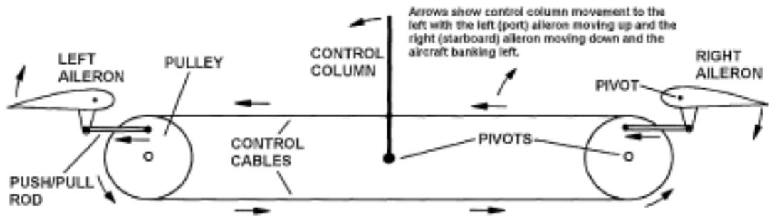
**Figure 4-5.** A simplified aileron control system
