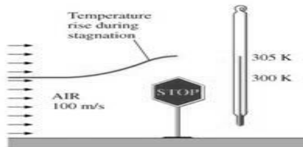
FIGURE 17-5 The temperature of an ideal gas flowing at a velocity V rises by V^2/2c_p when it is brought to a complete stop.
