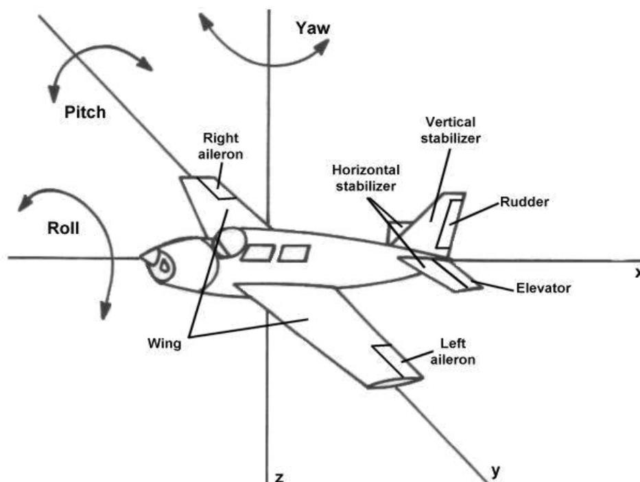
**Figure 4-1.** Motion of an aircraft about its axes
