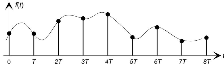
(ii) At each interval, the output sample  $y_n$  is computed, based on the history of the input and output, for example
