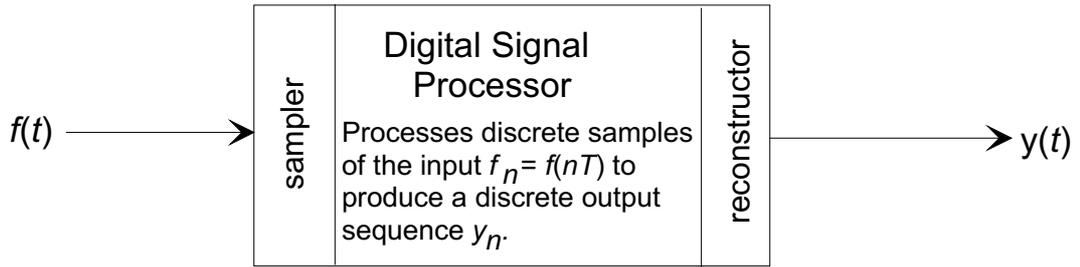
(i) The sampler (A/D converter) records the signal value at discrete times to produce a sequence of samples  $\{f_n\}$  where  $f_n = f(nT)$  ( $T$  is the sampling interval).
